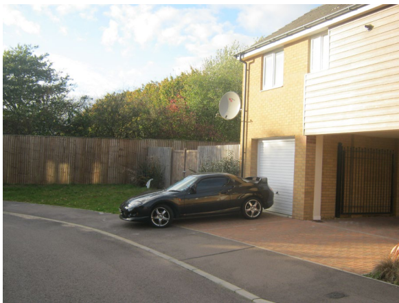
Figure 2: Example of unused garage with insufficient parking space in front of garage, resulting in the parked car over hanging the pavement.
